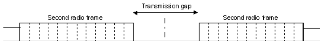
Fig. 4-5: Envelope of compressed mode signal with double-frame method
