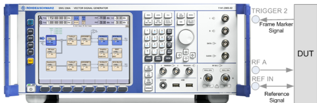
Fig. 6-1: Test Setup (example with R&S SMU)
